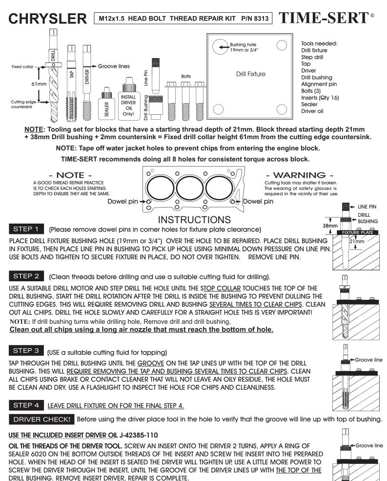
Check for the latest torque specifications before assembling the engine. Improper torque of the head can lead to thread failure.
